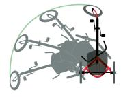
> Thanks to its geometry, a delta trike can turn on a dime – which can also be helpful when parking.
