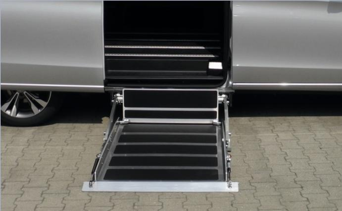
K90 in lowest position at the ground. Barrier folded down.
