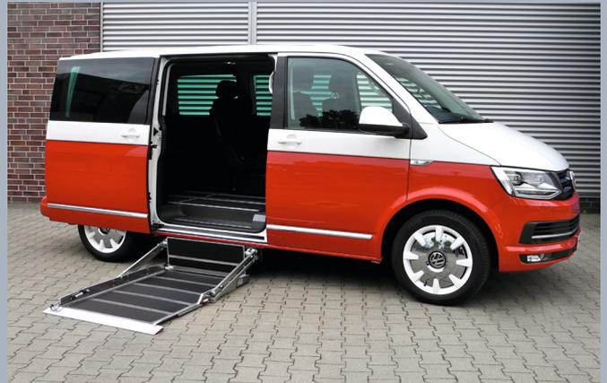
K90 in lowest position at the ground. Barrier folded down.
