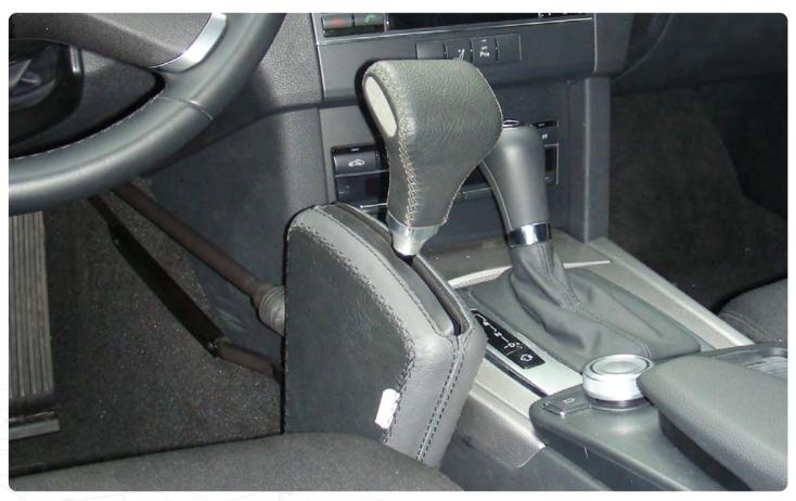
Unlike other floor mounted Levers on today's market the F1 EVO remains stationary, in order to avoid unwanted leg friction, we have designed it in such a manner that only the handgrip moves.
