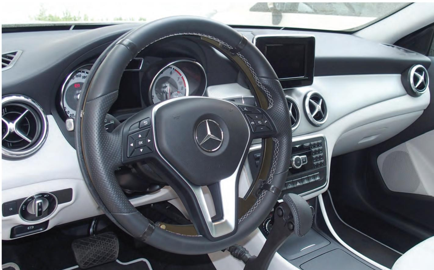
The only Rotating Ring Accelerator available on today's market, this unique design offers an effortless driving experience, simply rotate in either direction to obtain a smooth acceleration. Its unobtrusive design allows it to rest snugly behind the steering wheel allowing you the end user to maintain that familiar 10 to 2 hand position.
