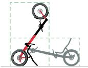
> Upright parking allowed! A delta trike can be parked with its front wheel in the air, which saves space indoors and is a real eye-catcher outdoors.
