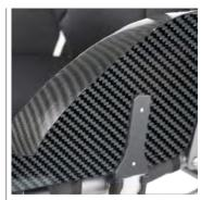
Lift out carbon fibre with fender
