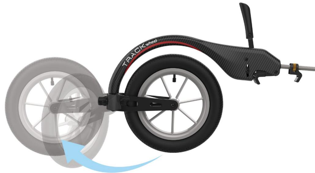
Turn your TRACK WHEEL outwards when attaching it and back inwards to the starting position for driving. You will find more details in the user manual.
