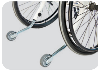
Anti-tipping supports prevent the truck from tipping over.
