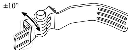
Fixed lateral supports are available for situations when a swing-away lateral is not required. Fixed lateral supports consist of shell bracket and pad.
