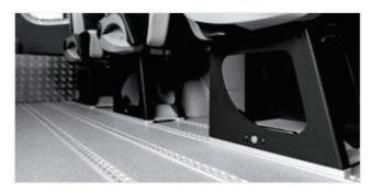
The TwinLock is a joined set of seat legs with a mechanism to secure the seat in the rails of the vehicle. It's easy to use and requires only one hand for operation. The low friction surface under the TwinLock allows seats to slide back and forth effortlessly in the tracks. Once in the locked position, the seat is tensioned into the tracks so there is no rattle.
