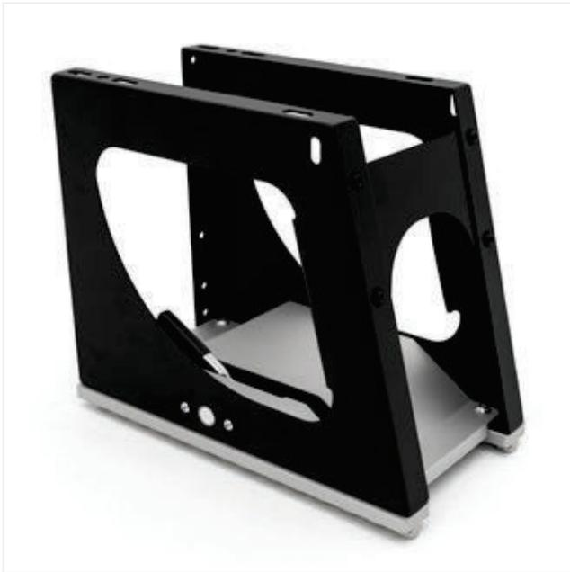
The TwinLock is a joined set of seat legs with a mechanism to secure the seat in the rails of the vehicle. It's easy to use and requires only one hand for operation. The low friction surface under the TwinLock allows seats to slide back and forth effortlessly in the tracks. Once in the locked position, the seat is tensioned into the tracks so there is no rattle.
