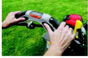
continuously varies output torque at the rear wheels to control ground speed. The transmission varies output torque by carefully controlling slippage in the cone clutch mechanism.
