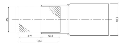
SP 960 Technical specifications Loading capacity 320 kg
