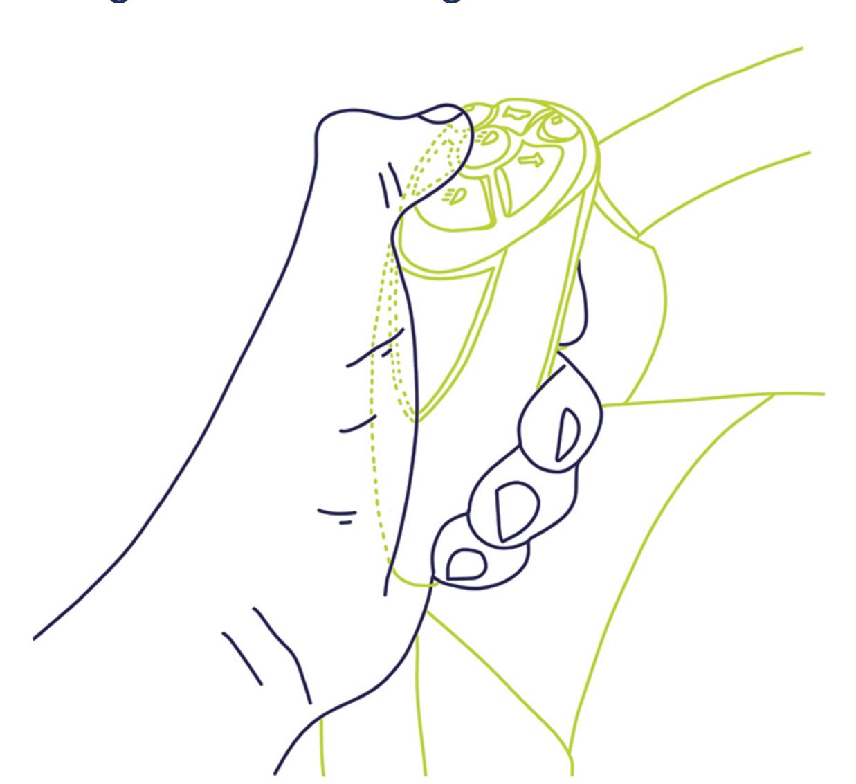
The LEHMDIS multifunction device has 7 buttons and can operate up to 10 functions:
