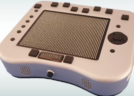
Tactile area 120 x 97 mm 10 point multitouch Windows 10 Mini-PC Bluetooth and wireless
