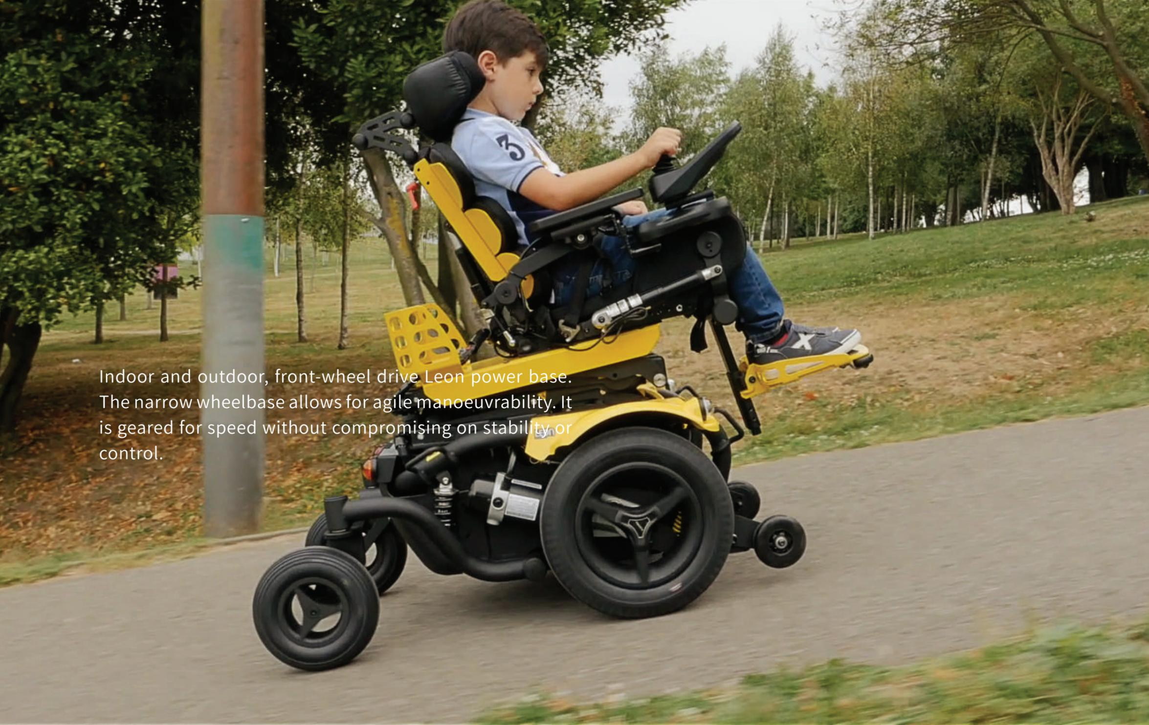
Indoor and outdoor, front-wheel drive Leon power base. The narrow wheelbase allows for agile manoeuvrability. It is geared for speed without compromising on stability or control.
