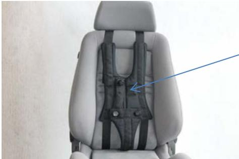
Place the belt chest cushion against the seat backrest, put shoulder belts with triangular assembly plate of the seat backrest. Plug the triangular assembly plate with the two lower belts and crotch belt in between the seat and backrest.
