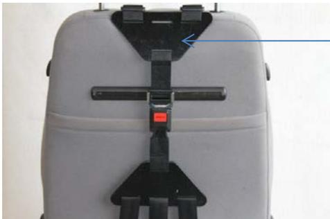
Place the triangular assembly plate high on the back of the backrest, close the lock and tighten the belt. This is done by tightening the belt on the triangular assembly plate.
