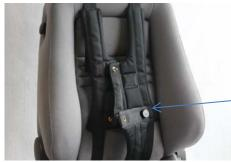
the person thereby ensuring the person in the seat with chest pad and crotch belt. Make sure the chest pad is positioned so it does not touch the neck. Then adjust the crotch on the back of the backrest in the lower triangular collection plate, the crotch belt should not be tight.
