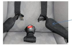
Ensure that relief cushions fit right where the belts have contact with the body
