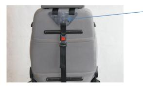
Place the triangular assembly plate high on the back of the seat backrest, close the lock and set the belt.
