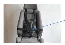
The harness is designed as a chest pad with fitted shoulder, hip and crotch straps with snap locks. All snap locks are located on the back of the seat backrest.
