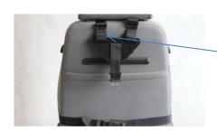
Place the triangular shoulder plate with shoulder straps high on the back of the seat so that shoulder straps cannot slide out on the side of the seat back.
