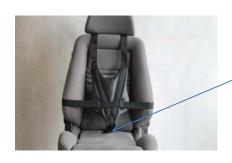
The crotch is inserted between the seatback and seat, the chest pad is placed on the seat, place the person's on the seat so the crotch is between the legs. Lift the chest pad to the person's chest and place the 2 shoulder straps over the back of the seat.
