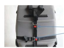
Take the crotch strap and lock it with the triangular shoulder plate. Then adjust the crotch strap to fit the person without tightening. The hip strap is placed around the seat backrest and locked. Adjust the hip strap to fit the person no more than there may be a flat hand between the backrest and the strap.
