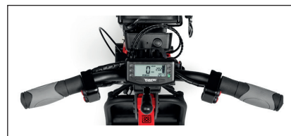
G&B handlebar option without levers for quadriplegics.
