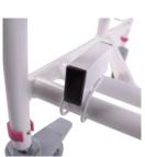
For users who are always being lifted, the forward tip may be undesirable. Therefore we offer a bracket that ensres that the chair cannot tip forward. The bracket is easily mounted on the front of the frame and stops the movement when the seat is in level position.
