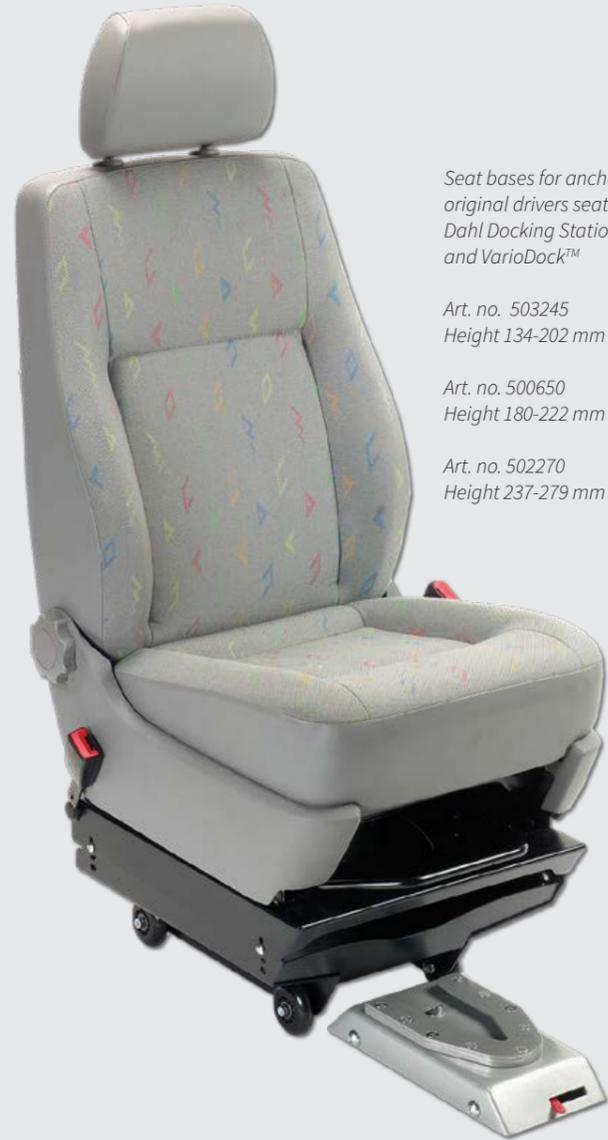
Seat bases for anchoring original drivers seats with Dahl Docking Station MK II and VarioDock™
