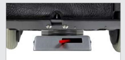
A lock plate and a spacer must be fitted under the wheelchair. When the wheelchair is maneuvered towards the docking station, it is guided into place by means of the lock plate and is secured automatically.
