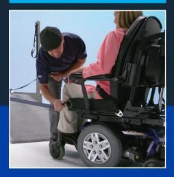
The operator releases the INQLINE Securement belts and attaches J-hooks to the wheelchair frame to secure the mobility device.
