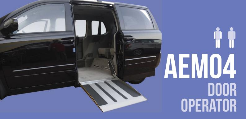
The door operator turns a manual sliding door into an electric powered door via an electric motor. You can control this movement by a switch, or a push-button handset or by a wireless radio control.
