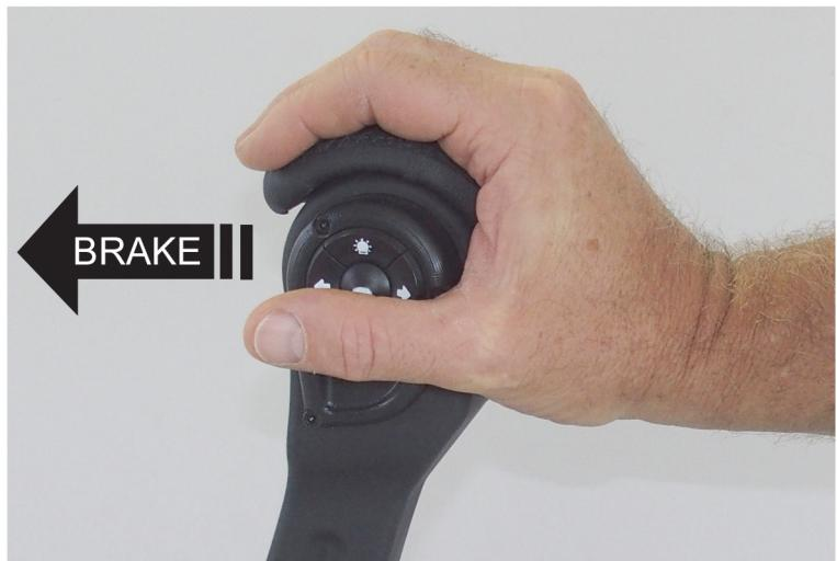
Acceleration is achieved by activating the electronic Half Moon trigger positioned strategically alongside of the ergonomic grip, the experience is light to the touch and thanks to our in-house IG Interface software acceleration can be programmed to suit individual needs, gradual or rapid... as is the case with all of our electronic solutions, acceleration is automatically inhibited once the brake is activated.
