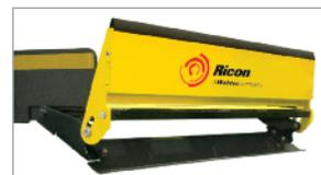
■ **Spring-Loaded Outboard Rollstop** – Outer rollstop features durable one-piece extruded aluminum design and mechanical actuator for smooth operation on widest range of surfaces.
