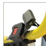
■ **Occupant Restraint Belt System** – Patented fully interlocked Ricon occupant restraint belt system combines with dual handrails, inner and outer rollstop barriers and side rails for industry-leading passenger security. Lift will not operate unless belt is securely fastened.
