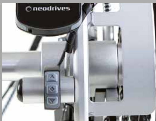
Control satellite for activating the pushing aid forwards with neodrives drive systems
