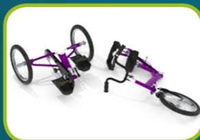
**Two Piece Frame Mechanism** ◊
