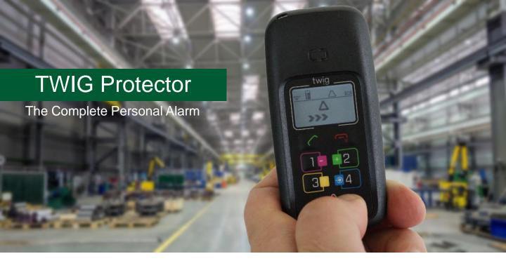
TWIG Protector is a complete 3G/GSM/GNSS personal alarm device designed to protect lone workers and those needing care.
