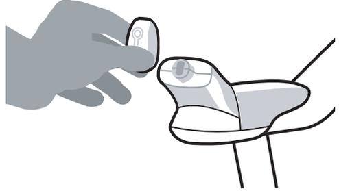
When the key is in the on position, the green power light on the armrest will come on.
