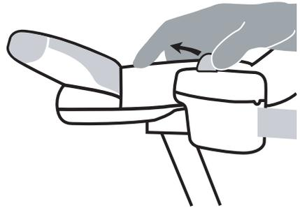
Swivel the seat back to its travelling position using either the standard swivel levers, or if you have an automatic swivel, the remote calling controls. You can fold the chair away if you wish.
