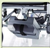
**Battery pack**Powerful battery pack with charging socket.
