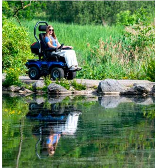
Originally designed for rural environments, with a rust-protected chassis and screws, the **P4** models adapt to many situations such as mud, snow, water (up to 10cm without submerging the motors), stones, etc.
