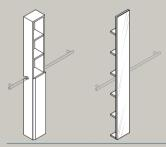
Container and mirror for anchorage on grab bar
