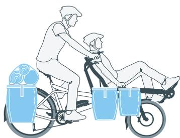
> With accessories like the Low Rider rack, which can carry up to four panniers under the front seat, the PINO is an ideal touring bike for both short and long excursions.
