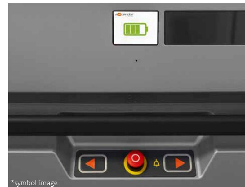
In the event of a malfunction, a **colour display** provides information about the cause and possible remedies. In this way, 80% of all maintenance cases can be avoided. The display also provides information about the current operating status at a glance.
