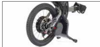
18" Wheel, ultra-grip tyre and aluminium double-wall rim.
