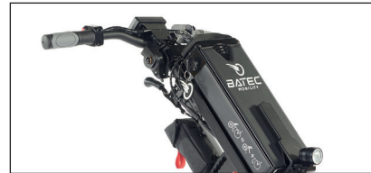
57,5 km* autonomy with 48 V - 748 Wh battery. Delivered with ultra-fast 3A charger.
